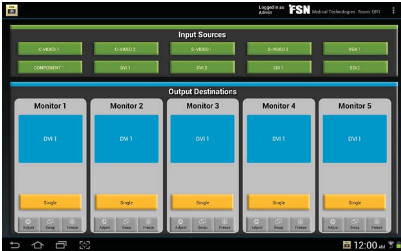
Sample dashboard is shown with 10 input sources (green) and 5 output destinations (blue).
